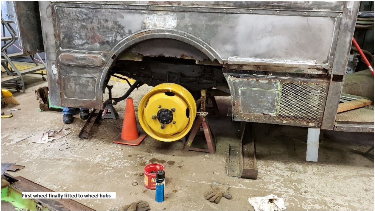
First wheel finally fitted to wheel hubs
